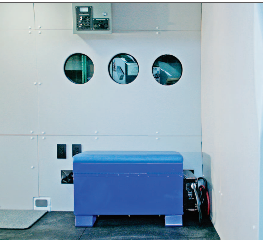
Porthole Windows and Battery Box
