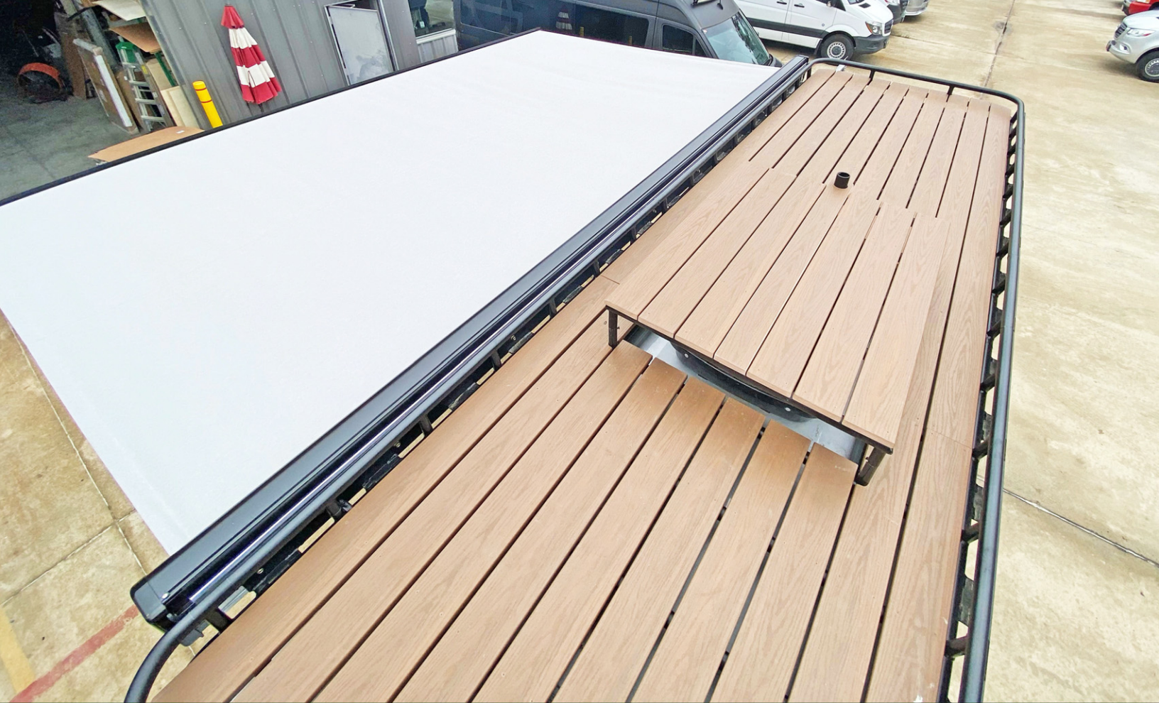
Roof Deck with Awning and Umbrella Mount
