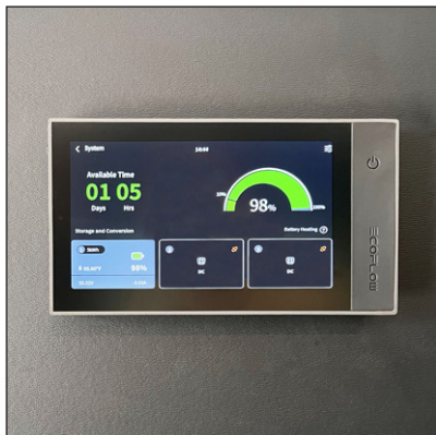
Power System Controller
