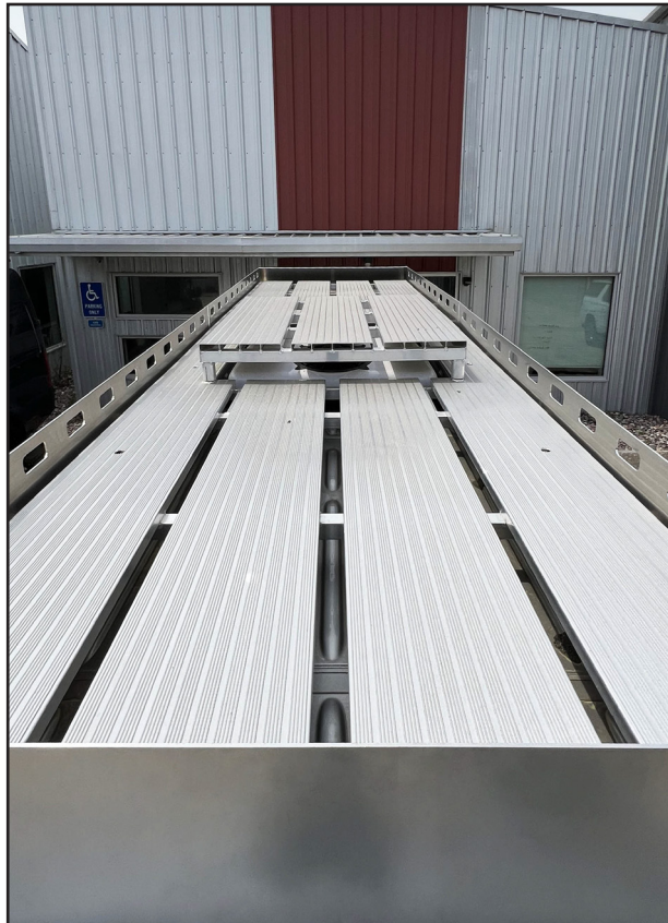
Custom Aluminum Roof Deck
