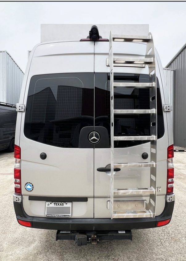
Ladder for Roof Access
